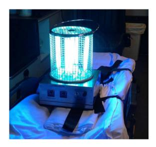
The EDU-435 has the highest UV-C output available for EMS. Rated UV-C energy output: 434 μW/cm² per second; 26,040 μW/cm² per minute @1 meter.
